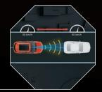
Adaptive Cruise Control is an advanced version of cruise control. It senses and monitors the road ahead and automatically accelerates/decelerates for maintaining a proper distance from the vehicle in front.
