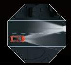
Intelligent Headlamp Control activates and deactivates the high beam, depending on the oncoming traffic and environment. Thus, preventing other road users from blinding due to high beam.
